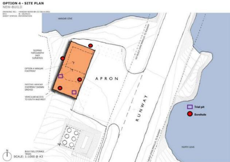
Figure 3-2 Proposed borehole locations for the Hangar SI
