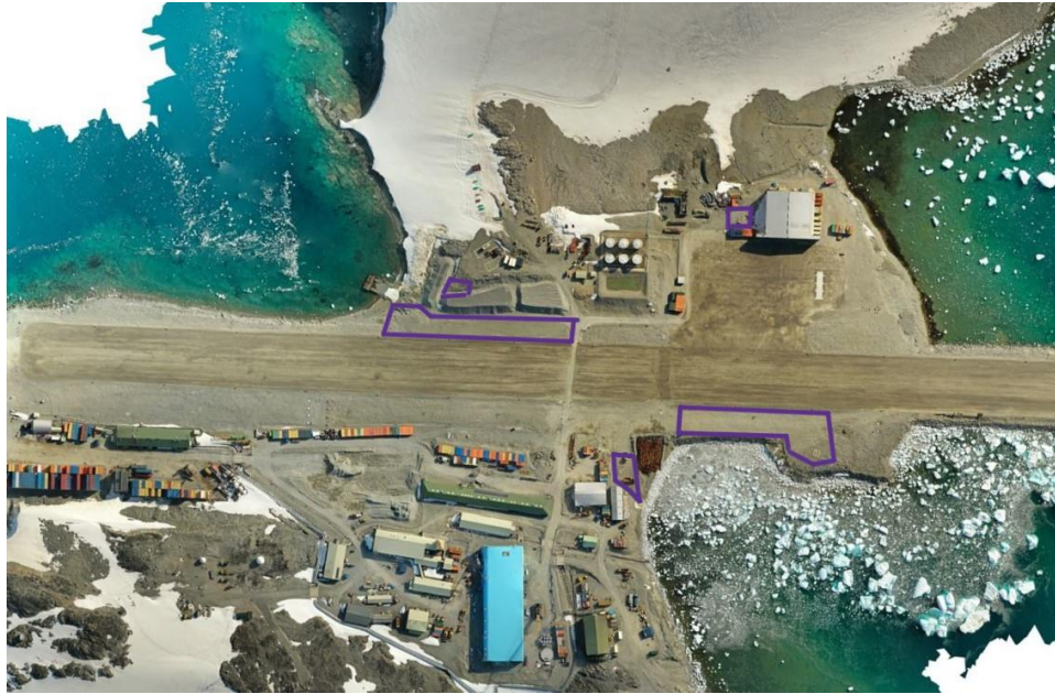
Image shown the proposed locations of the sources of aggregate for the runway verges.
