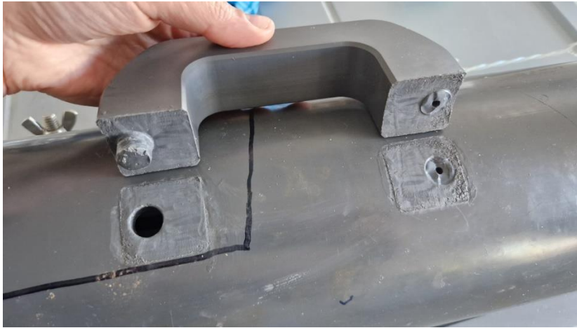
Figure 3: Photograph of the detached handle and 20 m Niskin bottle following deployment on the October patrol. Photograph from Carrie Gunn
