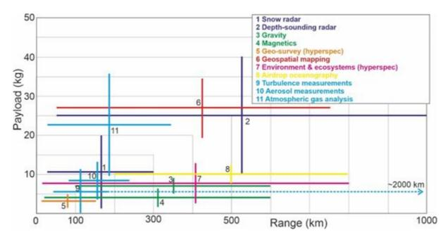
*Figure 2.2:* Expected range versus payload requirements for various science disciplines and sensors. Note in some cases deployment of multiple sensors on a single platform (increasing the payload) would be advantageous.
