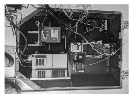
*Figure 4.1:* A series of broadband and hyperspectral imagers installed in the viewing hatch of the BAS Twin Otter aircraft by the NAEO. Each sensor is generally operated by an independent computer that has its own control and data storage requirements. Note boots at far left for scale. See Figure 2.1 for the actual aircraft this installation is hosted within.
