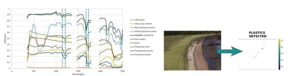
SWIR plastic features were found across plastic targets that shared composition. An algorithm for plastic detection was developed using those wavelengths.
