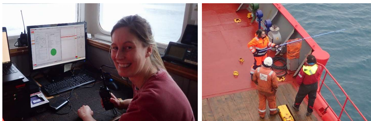
Figure 4. Kate Owen being trained in EK80 calibration (left). Tracey Dornan, Ryan Irvine and Bob Bosun using rods to manoeuvre the calibration sphere within the transducer beam during calibration (right).
