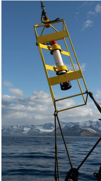
Figure 3. The CTD being deployed at the inshore end of ECB4.
