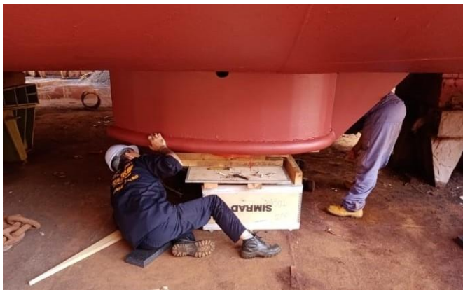
Figure 2. Acoustic echosounder being fitted to the vessel (left) and CTD being deployed from the vessel (right). Credits: Steve Brown and Martin Collins
